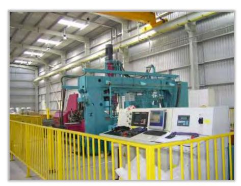
The KF Range of CNC plate machining centres are built for drilling and flame cutting of structural steel plate.
